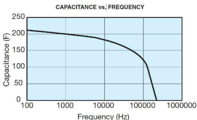
Tantalum capacitance and the frequency of the diagram
