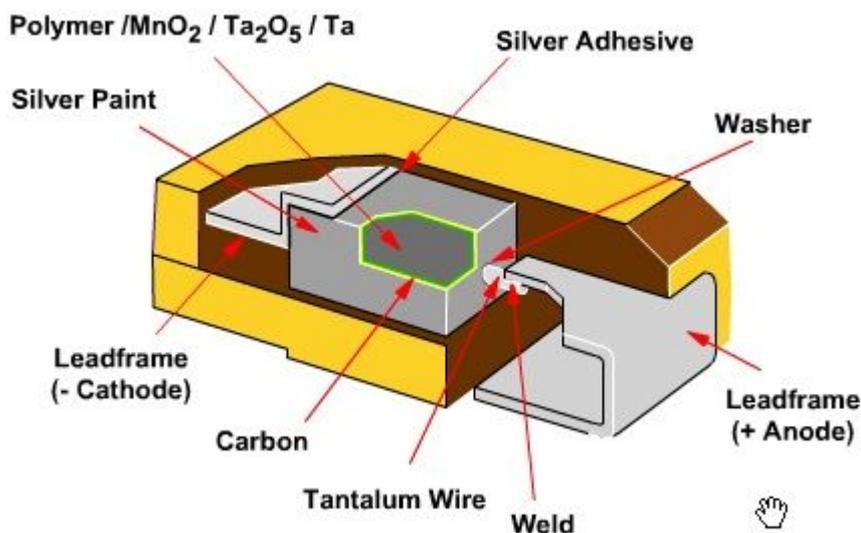
Basic solid tantalum capacitors by tantalum powder (the anode), oxide film (cannot exist independently of tantalum powder), manganese dioxide, silver powder, graphite, epoxy resin, lead.
